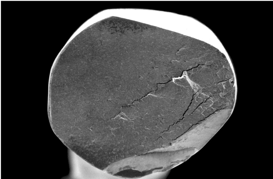
**Figure 3:** Typical fracture surface of a wire which has failed owing to tension-tension fatigue.
