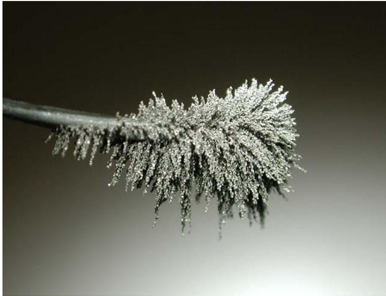
**Figure 4:** Using iron power to assess the degree of magnetism of a wire.
