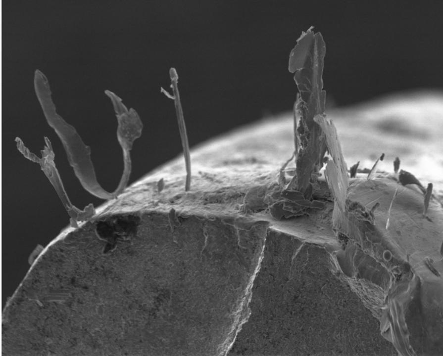
**Figure 5:** Poor quality SEM image of a wire fracture surface (tension-tension fatigue) owing to magnetism in the wire.
