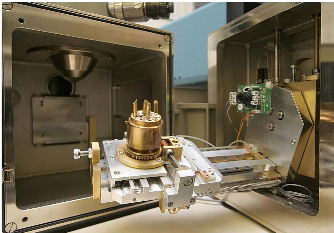
**Figure 2:** Detail of the vacuum chamber of a scanning electron microscope. (This can be seen closed at the left hand end in Figure 1.)
